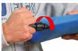
INSÉRER LE RACCORD - PUSH IN THE FITTING
